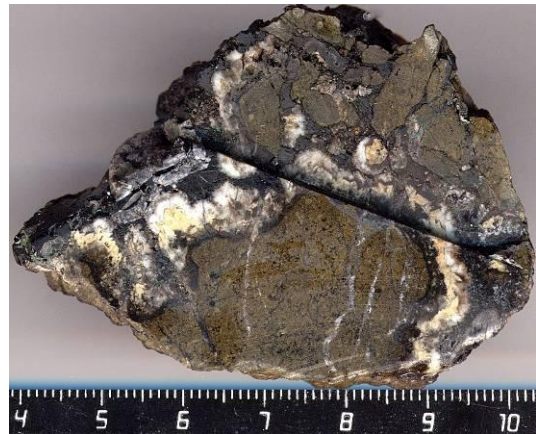
Fig. 2. Brecciated basalt cemented with bitumen
