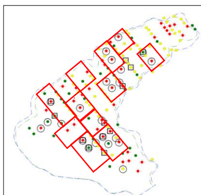
Fig. Relations between location of high injectivity wells with leaks and blocks with low reservoir pressure
